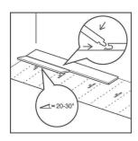
Turn the long side of the first panel of the second row into the already secured panel in the first row at an angle of 20-30°. Move the panel to be fitted slightly up and down and at the same time, exert some forward pressure. The panels will click together.
