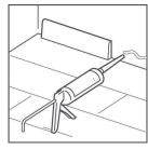
Inspect the final surface of the installed floor. Install base molding to the wall. Never attach the base to the floor itself. In places where profiles or base cannot be installed, fill the expansion space with silicone.
