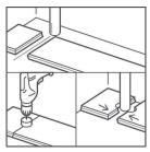
In rows where there is a pipe, make sure the pipe falls exactly in line with the short side of two planks. Take a drill bit with the same diameter as the pipe plus 1/2 inch (10 mm). Click the planks together on the short side and drill a hole centered on the joint between the two planks. Then install the planks.
