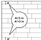
Measure the room before you start installing underlayment or flooring planks. Make sure that the last row of panels is at least 3 inches wide when finishing the installation. We recommend snapping a chalk line to ensure a perfectly straight installation.
