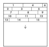
Continue the installation row by row towards the opposite side of the room. Always check each joint to ensure a good locking connection before continuing to the next plank. Press down gently with your thumb on top of every short end joint to ensure a good locking connection.
