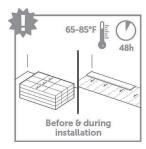
Always store and transport SolidTech Flooring on a flat surface in neat stacks to prevent warping. Never store the boxes upright or in moist, dusty rooms or in places with extreme temperatures. SolidTech Flooring must be acclimated in the room of installation between 65-85°F (18-30°C) for a period of at least 48 hours before installation. This temperature range should be maintained during installation and for at least 24 hours after the installation is completed.
