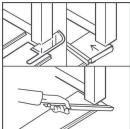
When the new flooring meets a threshold or a doorway, we recommend undercutting the door jamb. To secure the right cut, turn a plank upside down and place it on the floor up to the door frame. Then place a handsaw flat against the plank and simply cut through the frame. Remove the cut out and vacuum away debris. You can now secure the plank on the long side at the side of the door jamb. Use an installation tool pull bar to securely join the long and short joints.
