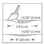
Any unevenness of more than 1/16 inch over a length of 3 feet (2 mm over a length of 1 m) must be leveled out. Remove bumps in the subfloor by sanding or scraping. The same applies to unevenness of more than 1/32 inch over a length of 8 inches (1 mm over a length of 20 cm). Use an appropriate leveling compound and check if a primer or sealer is needed with the supplier. In some cases, the use of an underlayment can avoid extra leveling of the subfloor.
