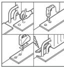
For a double pipe, drill a hole at each of the marked points that is equivalent to the diameter of the pipes plus 1/2 inch (10 mm). If located on the long side of the plank, make a 45° cut from each hole to the edge of the plank.
