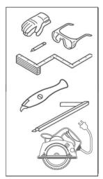
The following standard tools are needed: utility knife, tape measure, safety glasses, chalk line, speed square, tapping block, circular saw, gloves and a pencil. In addition to the standard tools, we recommend having a pull bar and carpenter's square available.
