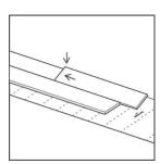
Then slide the third plank together horizontally. Slightly lift the plank to be installed by holding your hand underneath. Push the short side joint down gently with your thumb moving from the inner corner towards the outside until you hear a "click". Ensure the short side ends are closed by knocking gently on the short side click connection with the palm of your hand or tapping block
