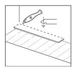
Start the first row with a whole plank. Cut off the long side tongue (end and edge) for the first panel. Position the cut edges adjacent to the wall.
