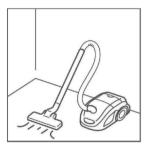
Make sure that the subfloor is dry, flat, stable, clean and free from debris, grease and chemical substances. If needed, scrape off and clean up old adhesives. Prior to installation, carefully remove all debris, sweep and vacuum. Repair surface imperfections and cracks. We recommend removing existing base trim and installing new moldings after installation of SolidTech Flooring is complete.
