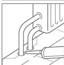
Then, using an appropriate glue along the cut edges of the piece you cut out, glue the piece in place. Be sure no glue comes between the cut out piece and the subfloor.
