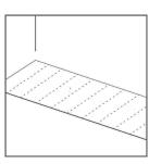
Begin in the left corner of the room. Install underlayment, if needed. Underlayment should be installed simultaneously with the floor installation. We recommend Mohawk ActiveSound Underlayment which helps ensure joint integrity, reduces sound, helps prevent indentation, and insulates and helps level the subfloor. SolidTech products with pad attached cannot be installed over separate underlayment
