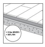
The moisture content of the concrete subfloor must be less than 85% relative humidity (RH test, ASTM F2170) or less than 5 lbs moisture vapor emission rate (MVER test, ASTM F1869). Always measure, record and keep your moisture content results.
