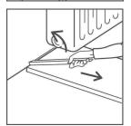
If it is difficult to tilt the planks (e.g. under radiators), use a pull bar installation tool to pull the planks together.
