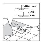
Make sure the subfloor is completely flat. Any joints of more than 1/8 inch (3 mm) in depth and 1/4 inch (6mm) in width should be leveled using an appropriate primer and leveling compound.
