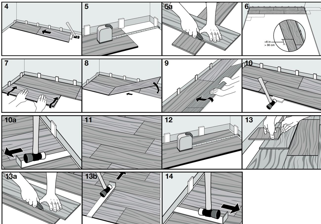
14. When the new flooring meets a threshold or a doorway, we recommend undercutting the door jamb. To secure the right cut, turn a plank upside down and place it on the floor up to the door frame. Then place a reciprocating saw flat against the plank and simply cut through the frame. Remove the cut-out piece and vacuum away debris. Slide plank under pre-cut door frame. Door frame should be cut so that a 1/4" (6 mm) gap is located from the edge of the plank under the casing to the wall.
