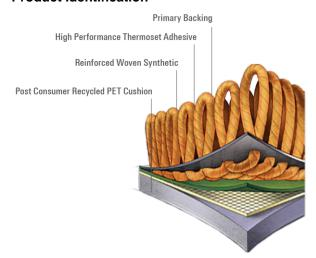
Unibond Plus Air is one of Mohawk's high performance commercial broadloom floor coverings with a nylon backing and face fiber. The Unibond Plus Air platform consists of various styles, colors, and patterns made with a nylon pile fiber layer and polypropylene backing. The pile fiber contains Type 6, 6.6, or Recycled Type 6 nylon with a PET attached cushion, which may be yarn dyed, solution dyed, or a combination of yarn and solution dyed.
