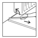
4. In rows where there is a pipe, make sure the pipe falls exactly in line with the short side of two planks. Select a drill bit with the same diameter as the pipe plus 1/2 inch (13 mm). Click the planks together on the short side and drill a hole centered on the joint between the two planks. Then install the planks.
