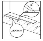
9. Then slide the third plank together horizontally. Slightly lift the plank to be installed by holding your hand underneath. Push the short side joint down gently with your thumb, moving from the inner corner towards the outside until you hear a "click". Ensure the short side ends are closed by knocking gently on the short side click connection with the palm of your hand or tapping block.
