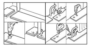
5. For a double pipe, drill a hole equivalent to the diameter of the pipe plus 1/2 inch (13 mm) at each of the marked points. If located on the long side of the plank, make a 45° cut from each hole to the edge of the plank.
