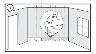
Start the second row from the right side. Cut and glue with silicone adhesive caulk the first plank. Fit plank by angling tongue into groove and wiggle into place. Use tapping block as needed. Drive a brad nail into each plank through the shallow area of the extended groove at each wall stud. (Figure 5)
