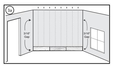
Drive a brad nail into each plank at each wall stud through the shallow area of the extended groove (see inset diagram). Take care that the brad nail heads are not raised, but also don't force them all the way through the groove. This will allow easy connection of the next row of planks. You must also place drywall screws every 16" into the wall studs or sill plate along the bottom edge of the first row of planks where they will be covered by the wall base. (Figure 4)
